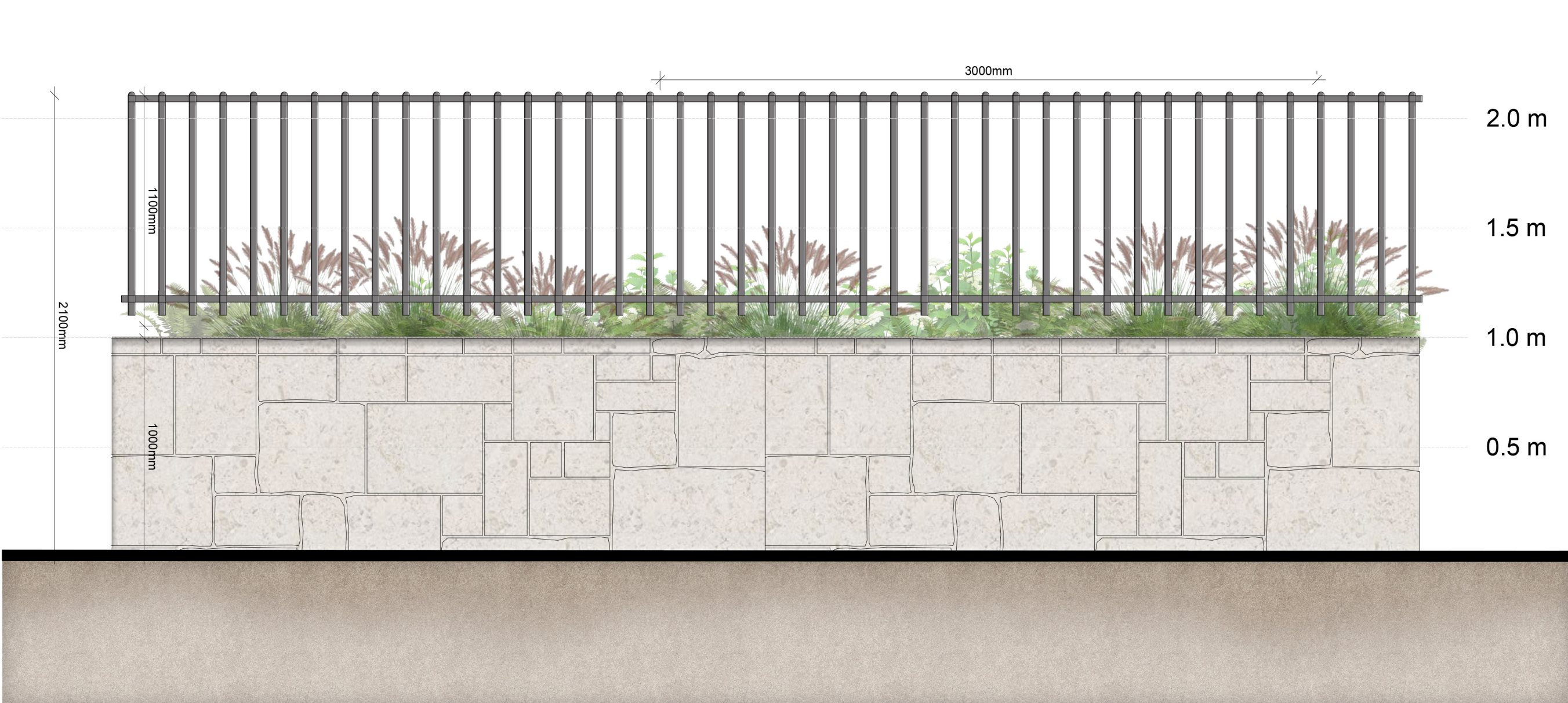
5 BT1a- Rubble stone wall and railings to 2.1m combined height- Elevation 400 scale 1:20 @A1
