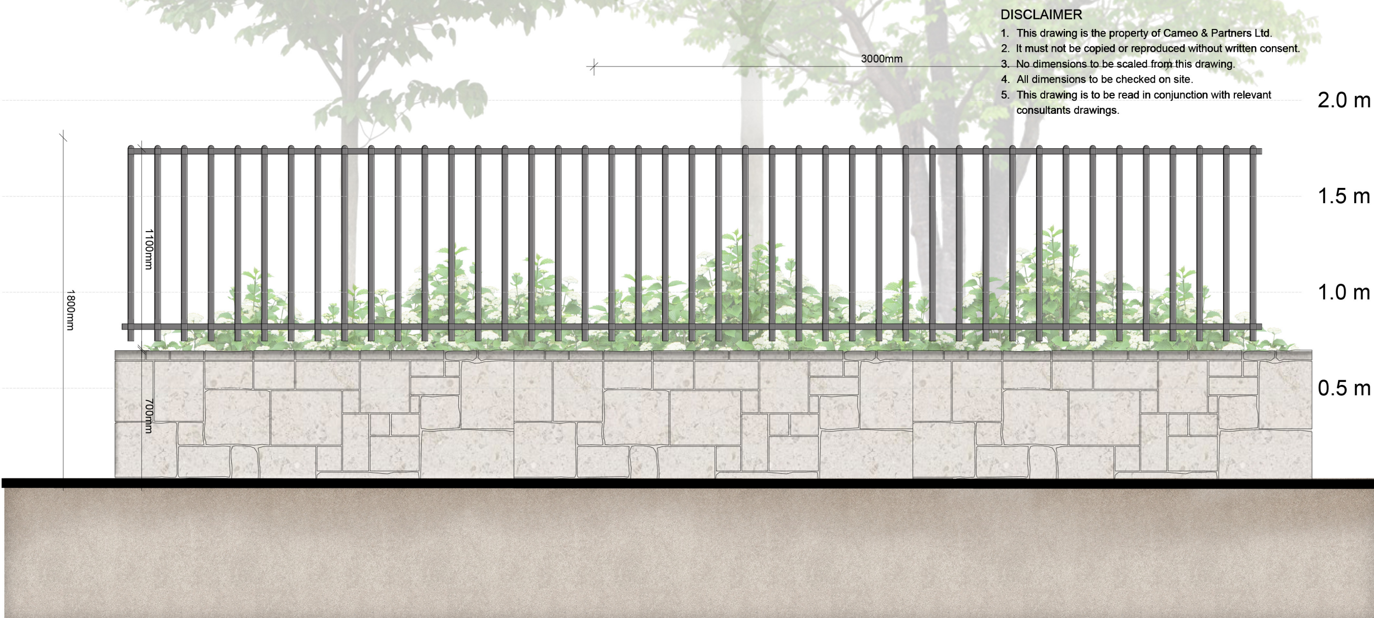
3 BT1-Low rubble stone wall and railings to 1.8m combined height- Elevation 400 scale 1:20@A1
